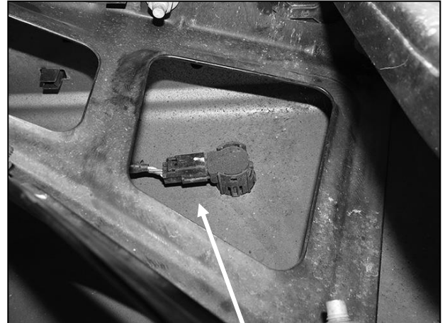
(Fig 6) Unplug the sensor first then remove the sensor from the mounting sleeve
